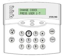
Enter the new 4-digit new code twice as per the display prompts. Three tones will be heard an acceptance of each command. A single low tone indicates that the procedure hasn't been completed and the process will need to be started again.
