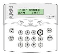
Similarly, if the down arrow key is pressed, the next most recent entry will be displayed. The up and down arrow keys may be used to scroll through the last 100 events in the event log. An error tone will be produced if an attempt is made to scroll outside either end of the event log.
