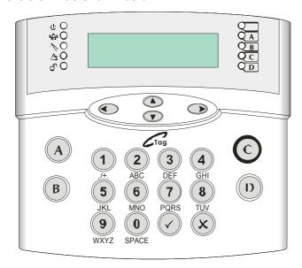
3. Press the (A) key to return back to the main screen of the log. Use the (A) and (A) keys to scroll through the log. Once completed, press the (B) key, 'Panel Log' will be displayed, press the (B) key twice to exit the manager menu.
