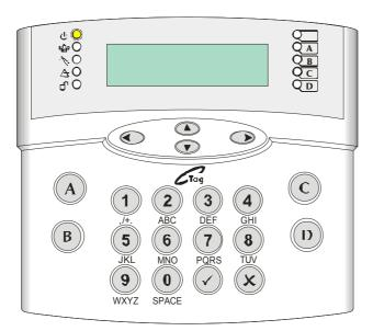
The power LED will flash indicating that a restore is required. Enter your engineering code. "All Faults Have Cleared" will be displayed. Press the key twice, 'Enter Code' will be displayed. Press the key to return to day mode.
